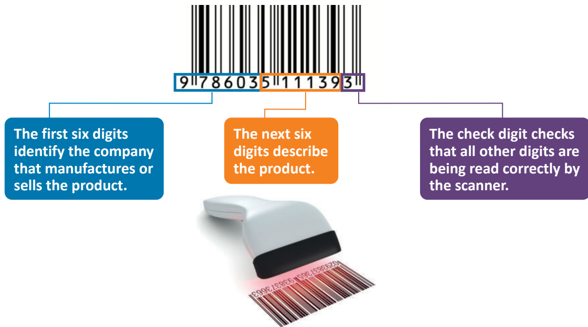
Figure 2.15: Example of barcode structure
